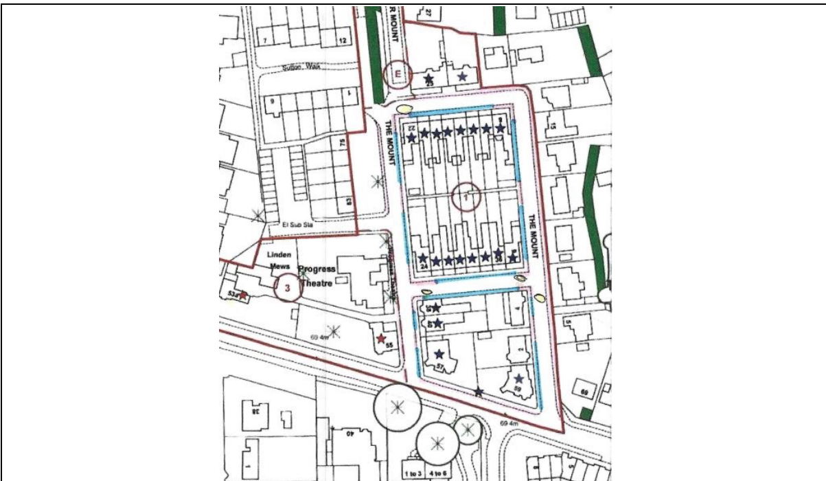
Figure 14 Diagram of location of stone (blue) and concrete (pink) kerbs, and original ironworks (circles) at The Mount (compiled by local resident)
