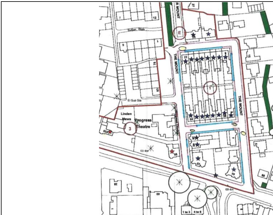
Figure 14 Diagram of location of stone (blue) and concrete (pink) kerbs, and original ironworks (circles) at The Mount (compiled by local resident)
